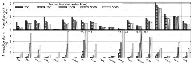
Figure 8: Performance overhead over native execution (top) and percentage of aborts (bottom) vs. transaction size (with 14 threads).
